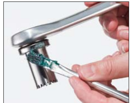
Figure 42. Greasing the bearings
